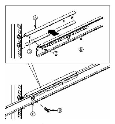
Figure 38: Attaching Rail Assembly to Front Bracket
